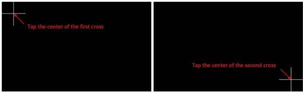
Note: After completing the calibration of the touch screen, you MUST execute save config command to save the calibration data.
