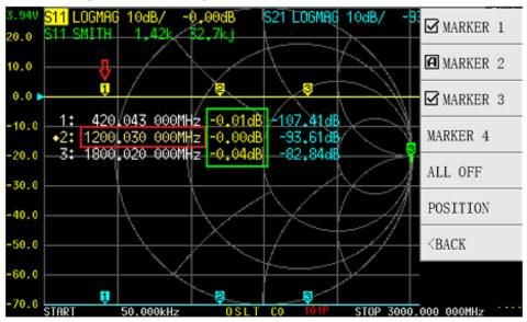
Tap on 【MARKER n】 (e.g., 【MARKER 2】) will open and activate MARKER 2, and an Amarker will appear ahead of "MARKER 2". Tap on another menu item (e.g., 【MARKER 3】) will open and activate MARKER 3, at this time, an Amarker will appear ahead of "MARKER 3", and the Amarker ahead of "MARKER 2" becomes ☑, which means MARKER 2 and MARKER 3 are both opened and MARKER 3 is current active.
